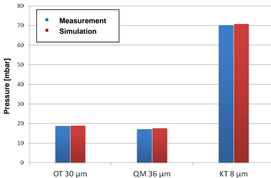
Fig. 5: Comparison of simulation results with measured values for different mesh types
