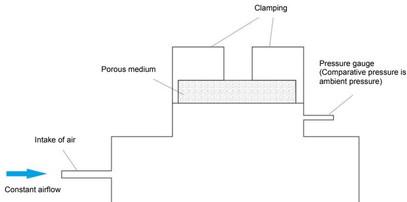
Fig. 1 Schematic diagram of the bubble point test
