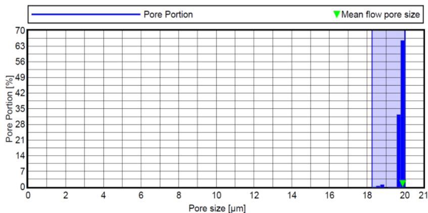
Fig. 7: Measurement of pore portion using improved method and adjusted capillary pressure constant
