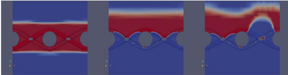
Fig. 4: Course of a bubble point simulation for an optimised dutch weave (OT 38)
