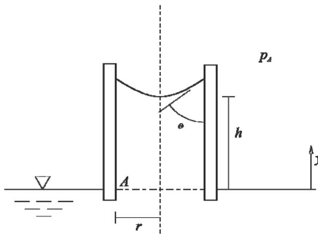
Fig. 2 Capillary action
