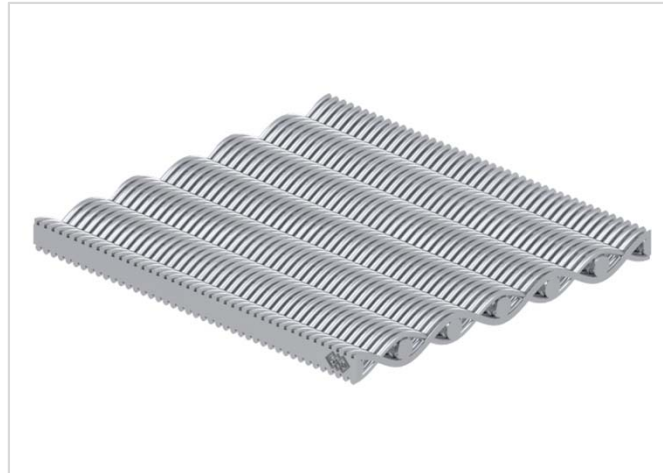
Picture 4: For each single weave type, like the optimized dutch weaves (ODW), a new capillary pressure constant has been calculated, in order to make a specific statement about the pore size.
